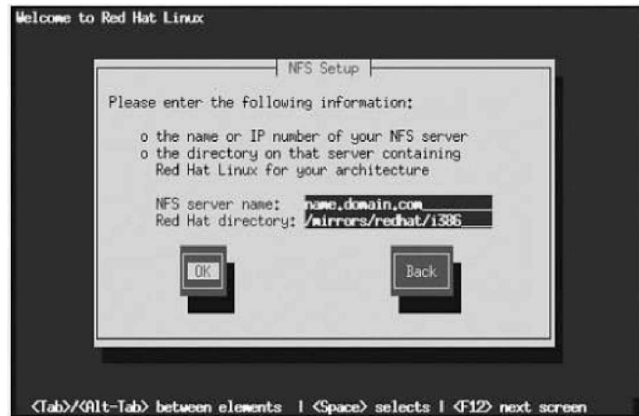
Gambar 5. Proses Instalasi Melalui NFS Server
